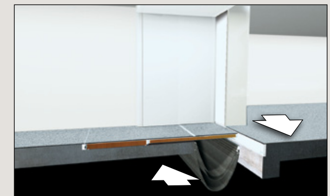
Lateral Shear The cab is attached to the fixed structure by means of a friction-free sliding track assembly to allow full lateral shear between buildings.
